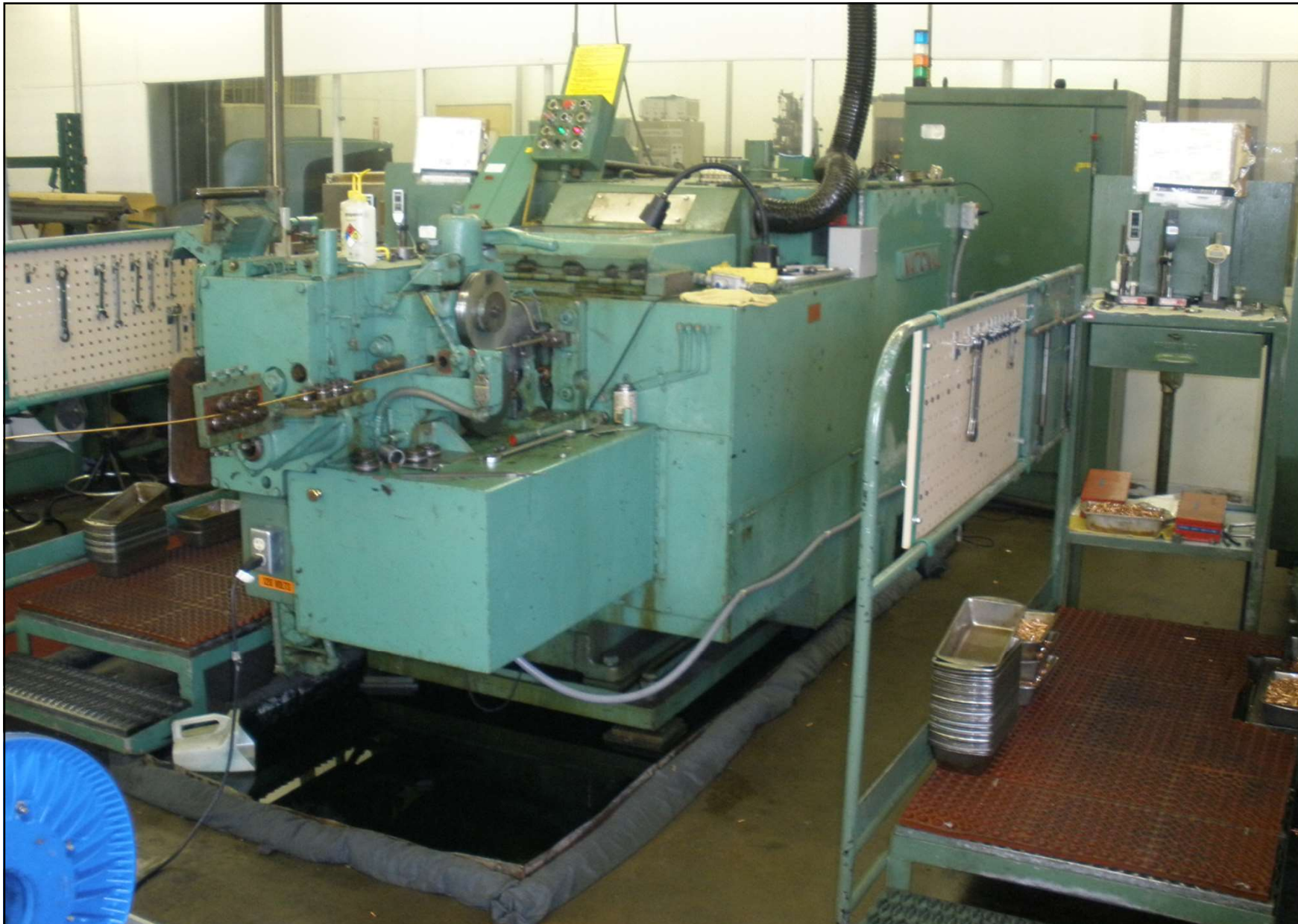
Example of oil filled equipment: machining mill and fluid reservoir
