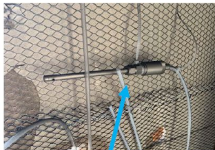
GT5000 Sample probe with integral 2 \mu m Teflon Filter fixed to mess on interior wall
