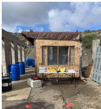
GT5000 setup outside the "reaction chamber" ~ 10ft Teflon sample tube
