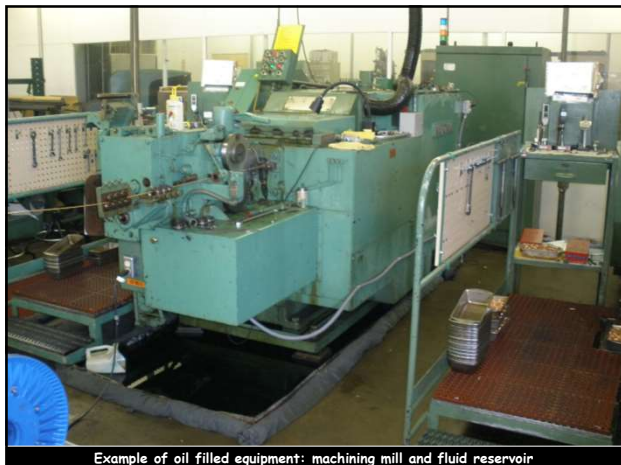
Example of oil filled equipment: machining mill and fluid reservoir
