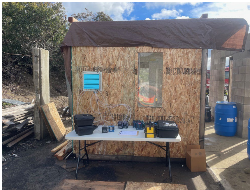
Photograph B: Side view of experimental shed showing plywood construction with a plexiglass window, a flap vent, and all EPA monitoring and sampling equipment being plumbed through the wall vent.
