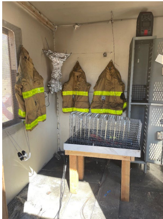
Photograph D: Inside experiment shed. Note the locker used to house equipment (inside or on top) and the raised tray to place test subjects on, this time with a mesh cage to prevent projectiles. Several firefighter “turnout” jackets were placed inside during experiments to be analyzed by a partner entity. EPA sampling and monitoring media is in the corner shielded by a tin foil barrier to prevent heat from melting tubing. Various vendor equipment can be seen throughout.
