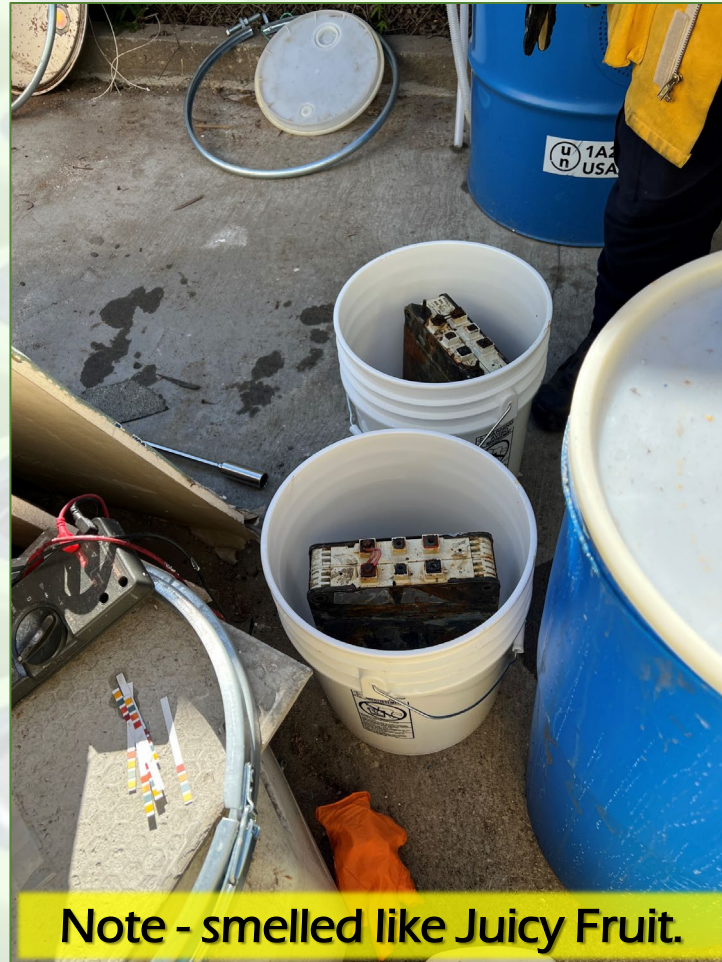
Verifying energy dissipation.
