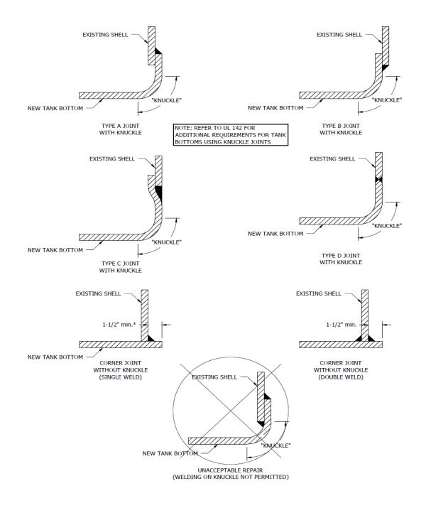
Single Fillet Weld of Tank Bottom
