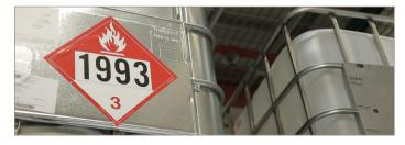
are permitted to be stored in these containers. However, the composite IBCs must be listed and labeled. The complete rules on what types of IBCs are allowed in buildings can be found in Chapter 9 of NFPA 30 (visit *www.nfpa.org/30* to access the chapters for free).
