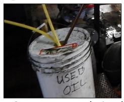
Used oil from 3 pumps were drained into a 5-gallon bucket through hoses. The container was continuously open as there was a hole for the hoses to enter the container.
