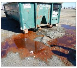
that was labeled "scrap metal". The leak was observed to be dripping at a steady rate for about one minute and did not show any signs of slowing down.
