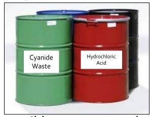
Incompatible wastes stored or accumulated adjacent to each other with no physical barrier for separation.
