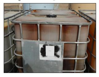
A polymer tote was observed with a crack and exposed top containing spent gas oil.
