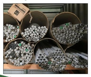
The inspector observed 11 cardboard boxes storing fluorescent lamps. The carboard boxes observed at the time of the inspection did not have lids or universal waste labels.
