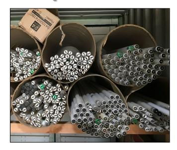
The inspector observed 11 cardboard boxes storing fluorescent lamps. Upon closer inspection, the inspector noted that three out of 11 cardboard boxes were storing lamps that exceeded the length of the box.
