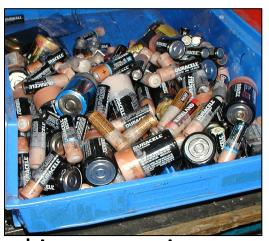
batteries were leaking corrosive waste and not labeled.
