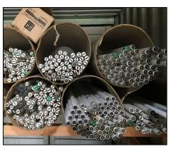
the inspector noted that three out of 11 cardboard boxes were storing lamps that exceeded the length of the box.
