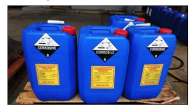
Incompatible wastes stored or accumulated adjacent to each other with no physical barrier for separation.
