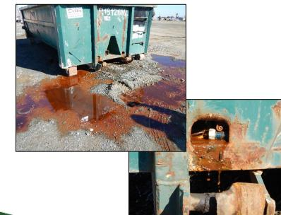
During an inspection, a leaking metal 30 cubic-yard roll off bin was observed. The liquid was observed to have been red/orange in color. The liquid was leaking from the bottom of a roll off bin that was labeled "scrap metal". The leak was observed to be dripping at a steady rate for about one minute and did not show any signs of slowing down.
