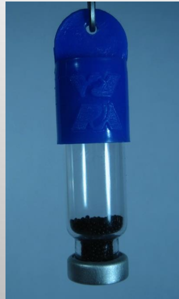
Diffusion on one end pass membrane (Waterloo Sampler)
