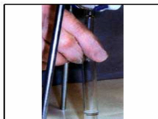
5. Drain solvent into test tube.
