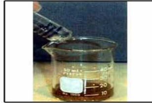
2. Snap ampoule, add solvent
