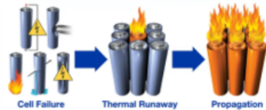
Figure 1: Diagram depicting a cascading thermal runaway event.
